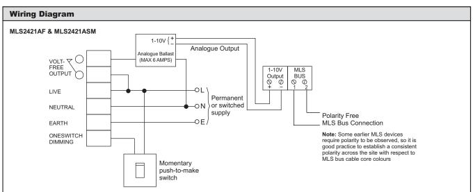
Relay outputs may be connected together in parallel to cover larger areas. The total load on all combined relay outputs must not, however, exceed 6 Amps as only one relay may be closed at a given moment.
