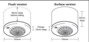
**Flush version:** Depth required behind ceiling: 62mm from front flange plus allowance for the minimum bend radius of the cable. Sinking box fits into 89mm diameter hole in ceiling tile or plasterboard ceiling. Note: If the sinking box is being fitted to a hard substrate such as metal, increase the hole size to 91mm. No access above the ceiling is necessary. The detector fits into sinking box with a simple bayonet action thus concealing the fixing screws.
