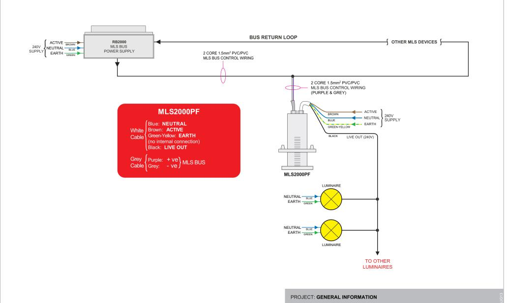
WIRING DIAGRAM: MLS2000PF DETECTOR
