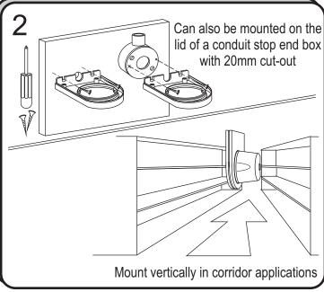
Offer the detector up to the WMK and twist into place
