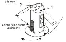
Carefully bend the plasterboard fixing springs down and hold the detector, FR64 and springs (once bent into position), as one, from below. Care must be taken not to release the springs in this position as they are under pressure and may detach from the detector. Feed the detector and cable through the 64mm hole until the assembly is flush with the ceiling.
