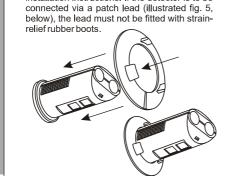
Insert the plasterboard fixing springs into the two cut-outs at the rear of the detector. They will be held in place by the plasterboard ceiling once installed. Please note that in the drawing below, spring '2' will locate around the support pillar on the FR64 when fitted in the ceiling. The FR64 and fixing spring must be aligned this way.
