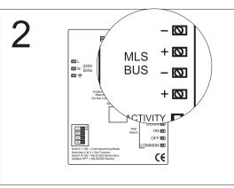
2. MLS Bus connections. Do NOT connect mains to the MLS Bus. Polarity must be maintained.
