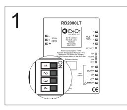
4-way DIL switch. All switches set to OFF by default. Switch 1 enables commissioning mode; Switch 4 determines bus type. Switches 2 and 3 - no function.
