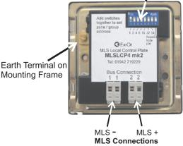
**NOTE:** The MLSLCP consumes two 'nodes' on the MLS Bus (max 200 with RB2000 Bus Power Supply; max 100 with RB2000LT Bus Power Supply 'Lite').
