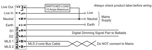
Note: A means of disconnection must be incorporated into the fixed wiring in accordance with the current wiring regulations.
