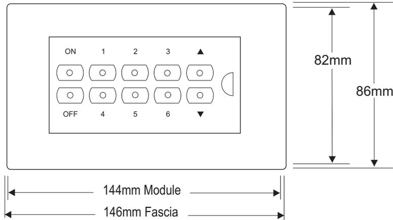
The module's enclosure and its supporting frame are designed to attach to the front of any standard Two-Gang Box, sinking, dry-lining or surface mounting, with a minimum depth of 30mm.
