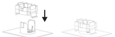
3. Align the oval on the front face of the sensor with the opening in the bezel and clip the sensor into place.
