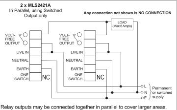
Relay outputs may be connected together in parallel to cover larger areas, however the total load on all combined relay outputs must not exceed 6 Amps. DO NOT CONNECT DIMMING OUTPUTS TOGETHER.
