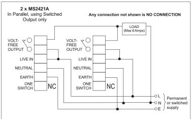
Relay outputs may be connected together in parallel to cover larger areas, however the total load on all combined relay outputs must not exceed 6 Amps. DO NOT CONNECT DIMMING OUTPUTS TOGETHER .
