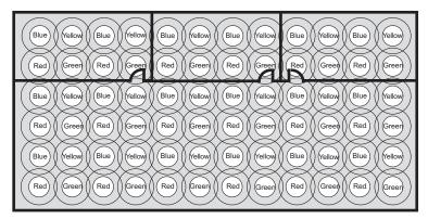
**Note:** Should it be necessary to order additional detectors for an existing installation and specific colour-coded detectors are needed, please add the following suffixes to the part number: Y = Yellow, B= Blue, G= Green, R = Red. (There is normally no need to specify the colour codes, as orders are dispatched with a suitable colour code mix.)
