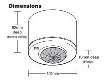
MINIMUM MOUNTING PITCH (SPACING): 0.5 x mounting height (when utilising the photocell)
