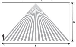
MINIMUM MOUNTING PITCH (SPACING): 0.5 x mounting height (regulating mode only - see note under 'Fixing')
