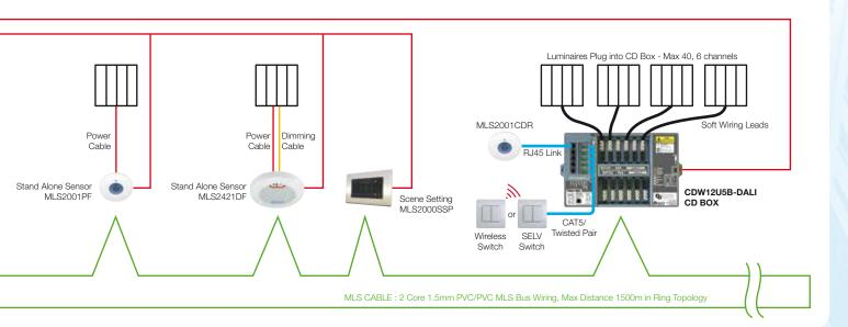
The sensors also communicate with other buildingwide sensors to achieve common and building zones. For example, adjacent corridors (common zone) can be illuminated when surrounding rooms are occupied, and the reception area (building zone) can also be luminated if any area in the building is in use.
