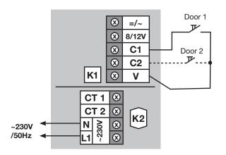
Power Supply Start Sound 230V~ (50HZ) 8-12V~
