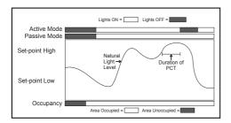
lights are now switched on again, completing the acknowledgement "blink". The OK button can now be released. Note that the difference between the two Set-point values, the Switching Hysteresis, is equal to the contribution to total light made by the controlled luminaires. This is the ideal amount of hysteresis to prevent oscillation without compromising control accuracy.
