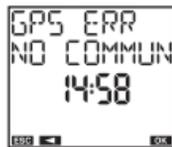
GEO-1 module is not properly connected to memo BUS.
