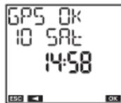
GEO-1 module has hooked a sufficient number of satellites for a correct synchronization.
