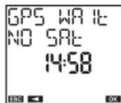
GEO-1 module has not hooked a sufficient number of satellites for a correct synchronization.
