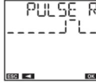
Turning on at sunrise for a settable short duration (pulse, max 59 seconds).
