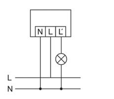
Standard operation with additional connection of external loads
