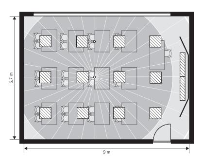
Planning example of installation of classroom set 1 in a typical classroom approximately 60 m<sup>2</sup> in size. Room height 3 m, planning criterion 500 lux (suitable for adult education) at a working level of 0.75 m.
