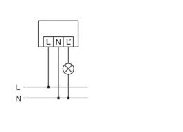
Standard operation with the additional possibility of switching on by hand. Note: with AL U 180 special functions can also be activated.
