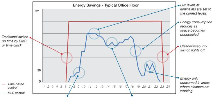
Energy consumption increases as space becomes occupied Daylight harvesting combined with occupancy control
