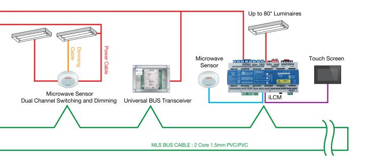
control functionality. Sensors can be manually overridden with scene select panels and/or local switches.
